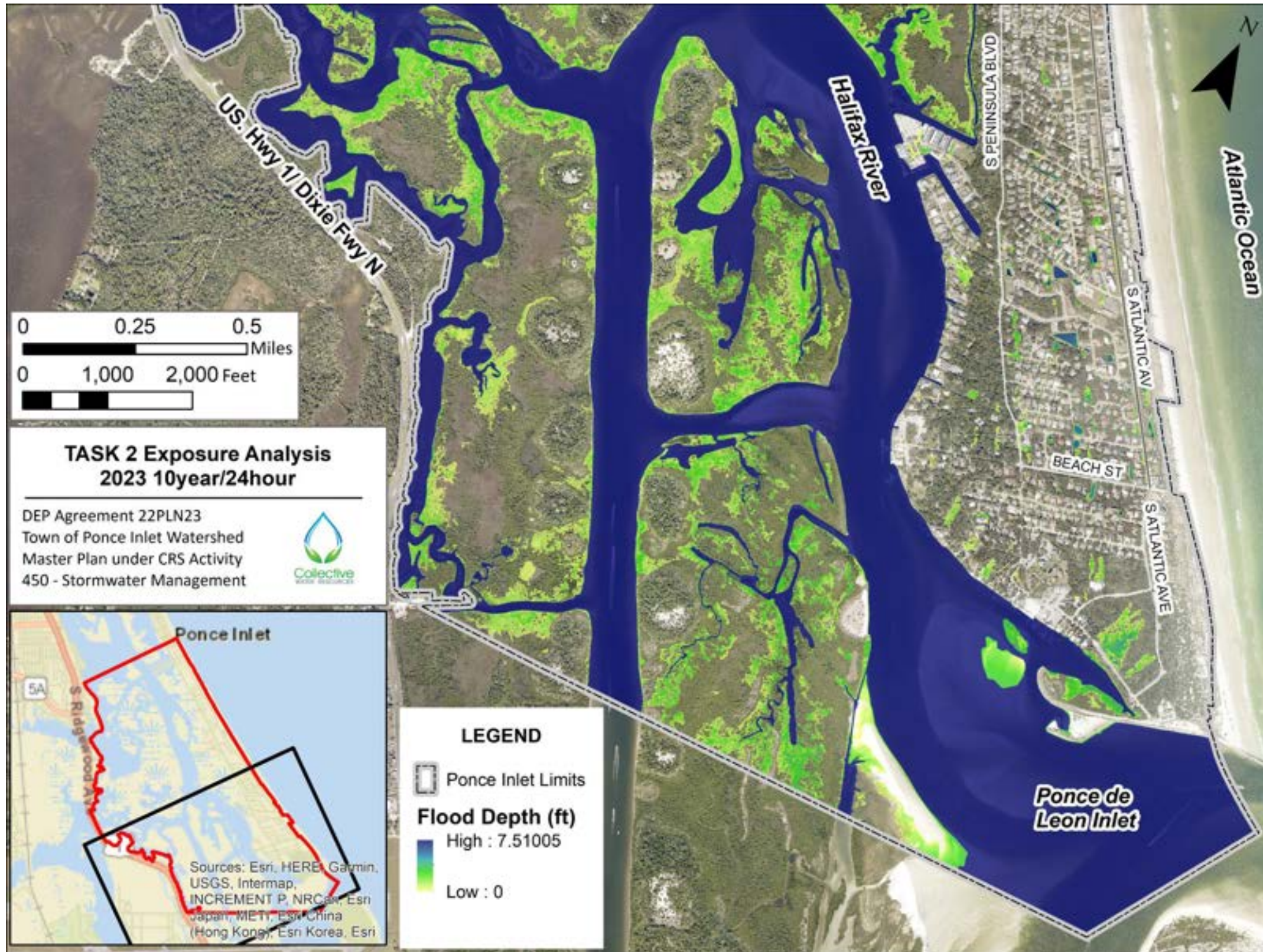
Figure F2 Stormwater Exposure 2023, 10year/24hour design storm South
