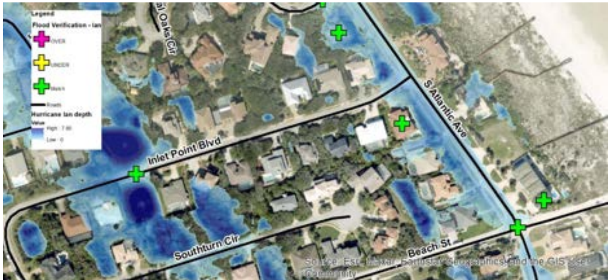
Figure 16. Simulated Hurricane Ian Flooding for Inlet Point Boulevard Area
