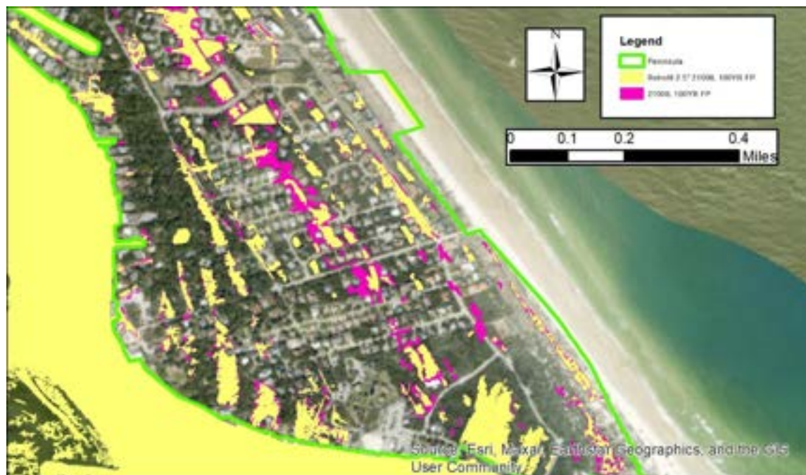
Figure 36. 2100 IL Floodplain with 2.5-Inches of Retrofit Retention/Storage
