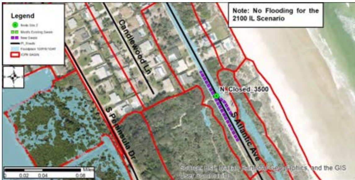
Figure 22. Site 2 Ponce Preserve Park, Swale Flooding and Reduction
