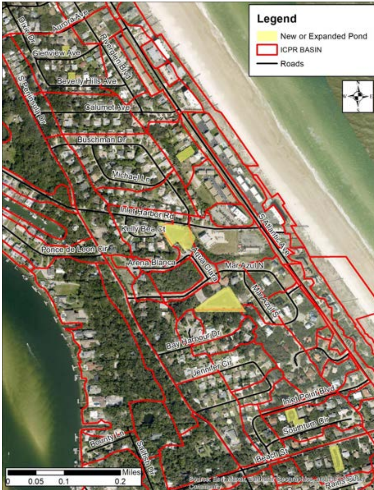
Figure 42. Potential New and Expanded Stormwater Storage Facilities
