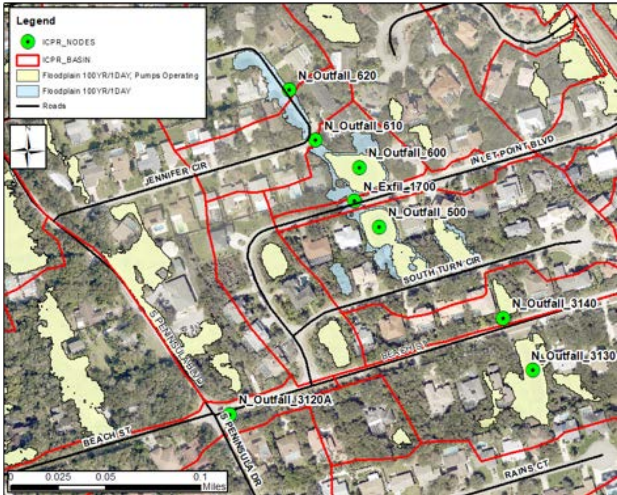
Figure 43. Pumping Alternative Floodplain Improvements, Current Conditions 100year/24hour storm
