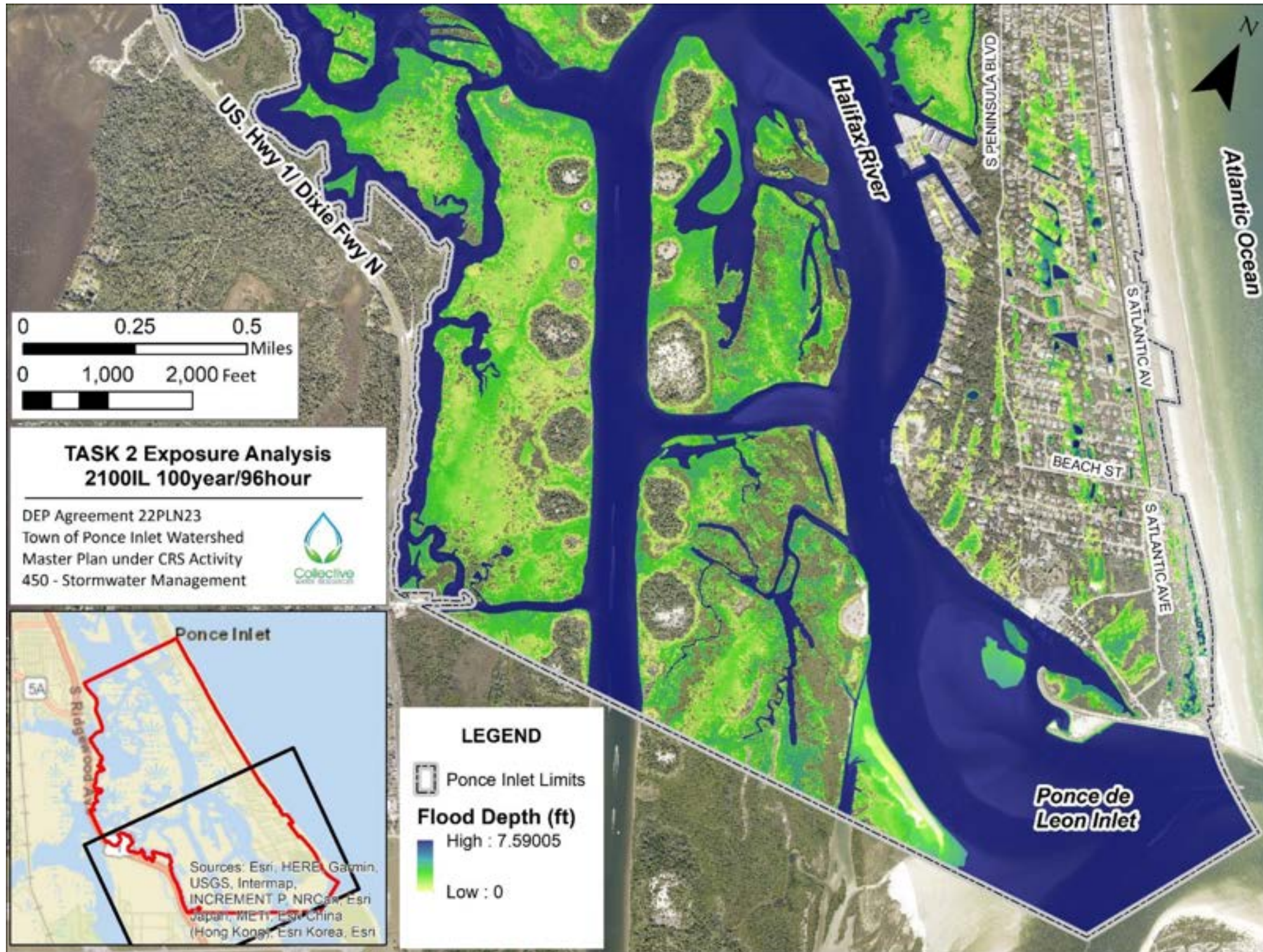
Figure F28 Stormwater Exposure 2100IL, 100year/96hour design storm South
