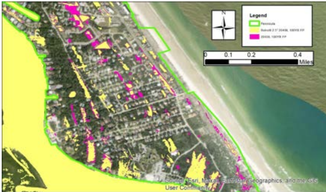
Figure 34. 2040 IL Floodplain with 2.5-Inches of Retrofit Retention/Storage
