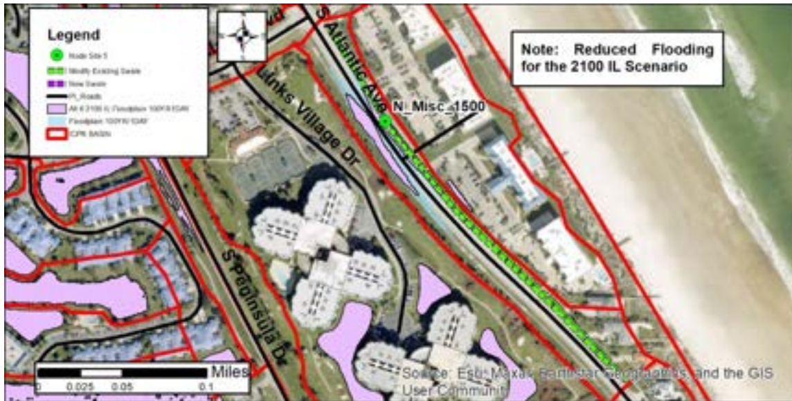
Figure 25. Site 5 South of Harbour Village Boulevard Swale Flooding and Reduction
