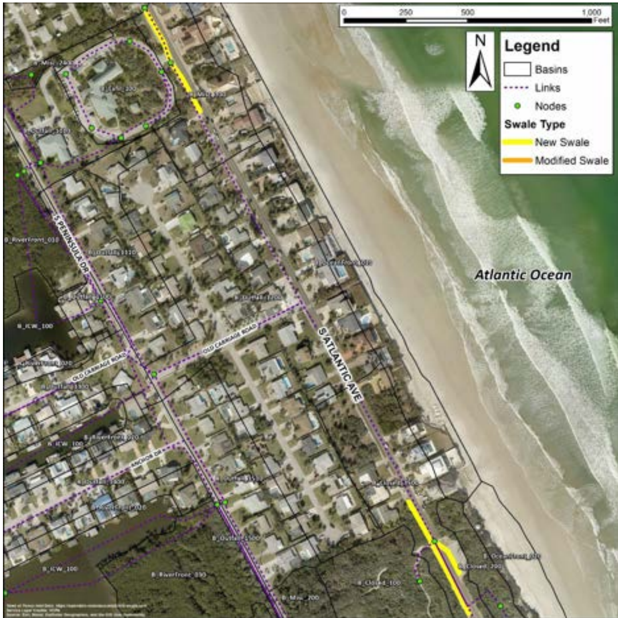
Figure 39. S Atlantic Avenue New Swale Locations Between Major Street and Ponce Preserve
