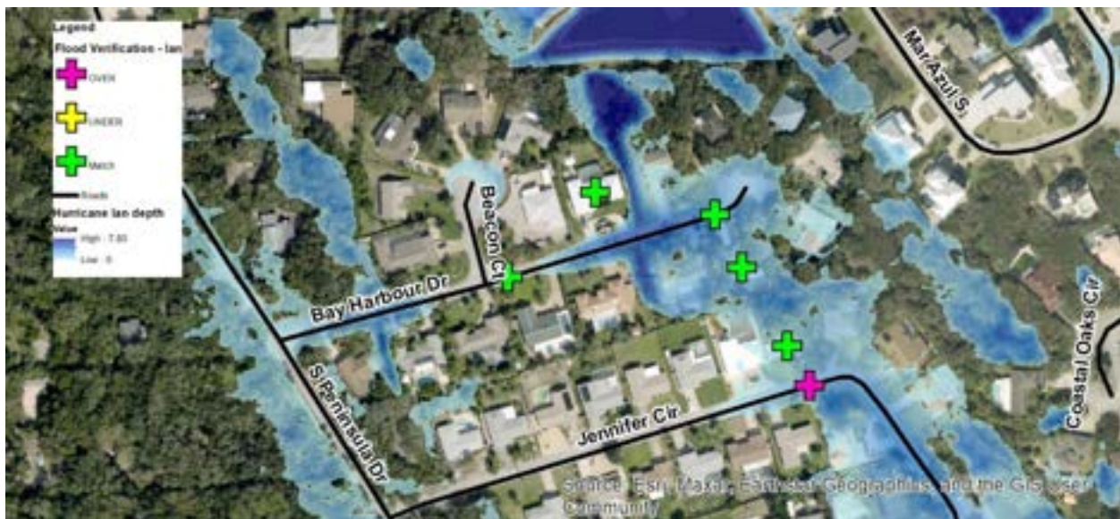
Figure 10. Simulated Hurricane Ian Flooding for Bay Harbour Drive Area
