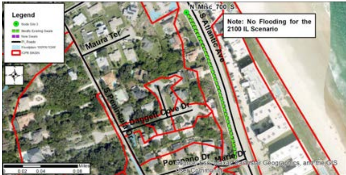
Figure 23. Site 3 North of Marie Drive, Swale Flooding and Reduction
