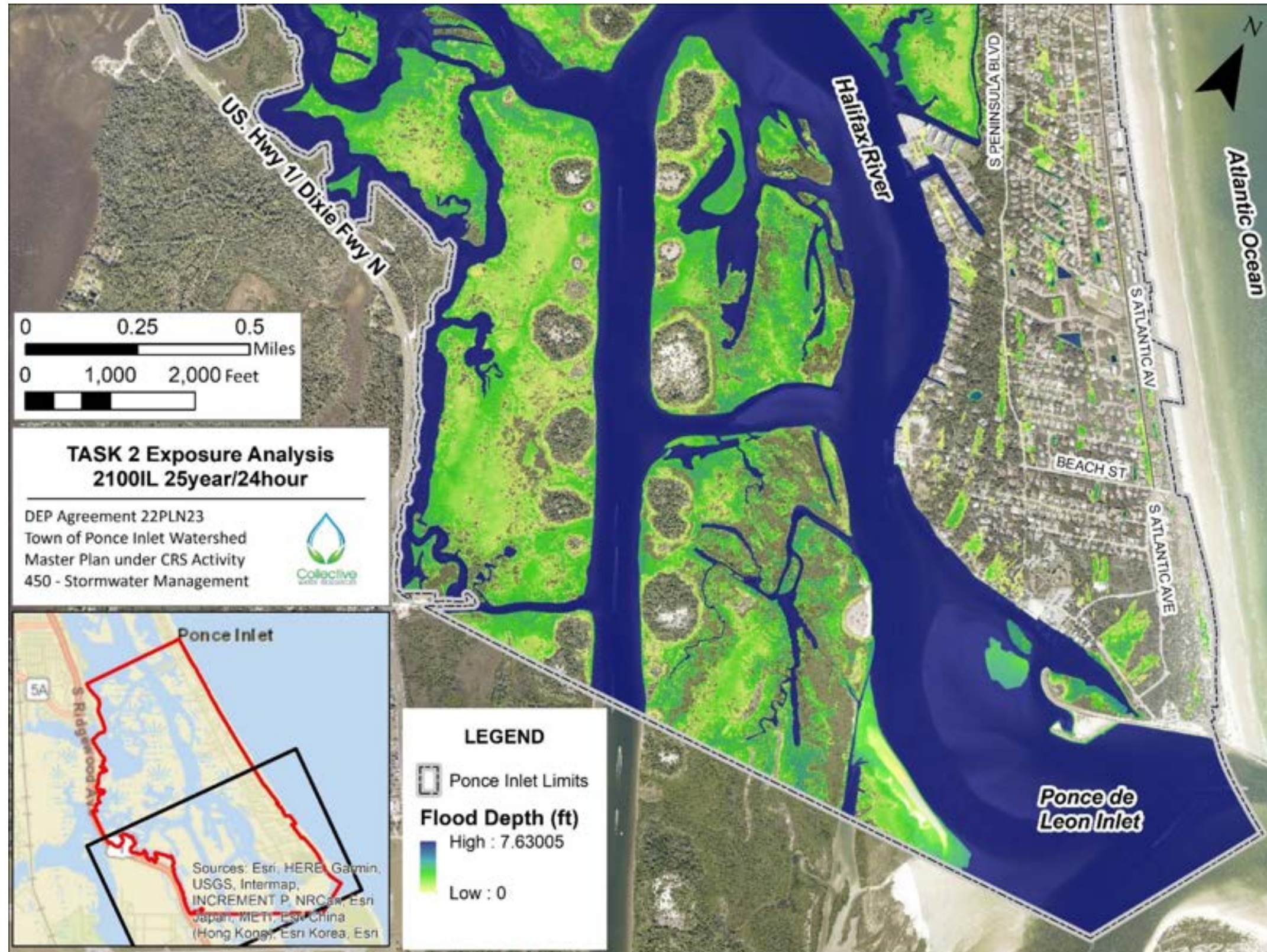
Figure F22 Stormwater Exposure 2100IL, 25year/24hour design storm South
