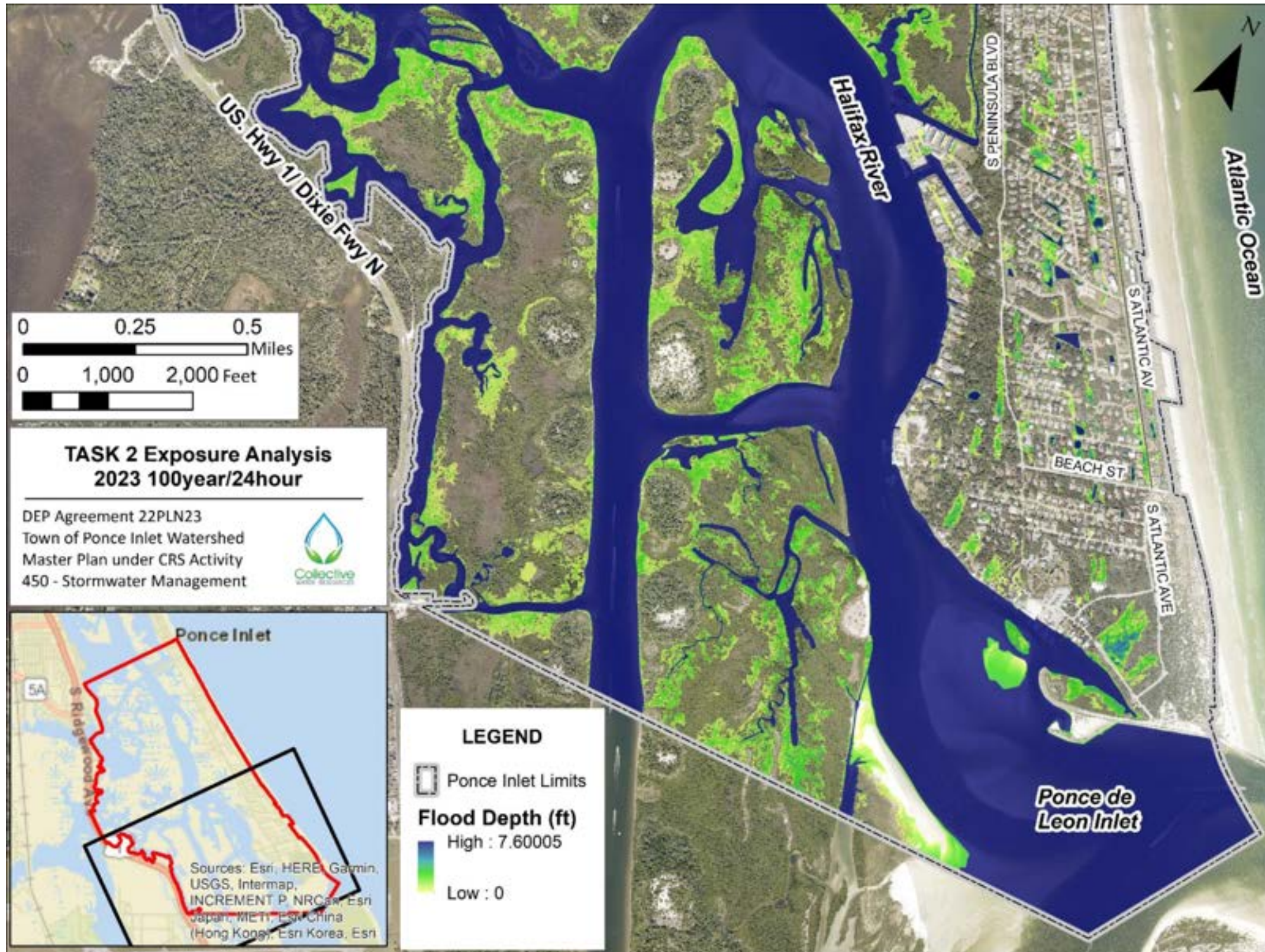
Figure F8 Stormwater Exposure 2023, 100year/24hour design storm South
