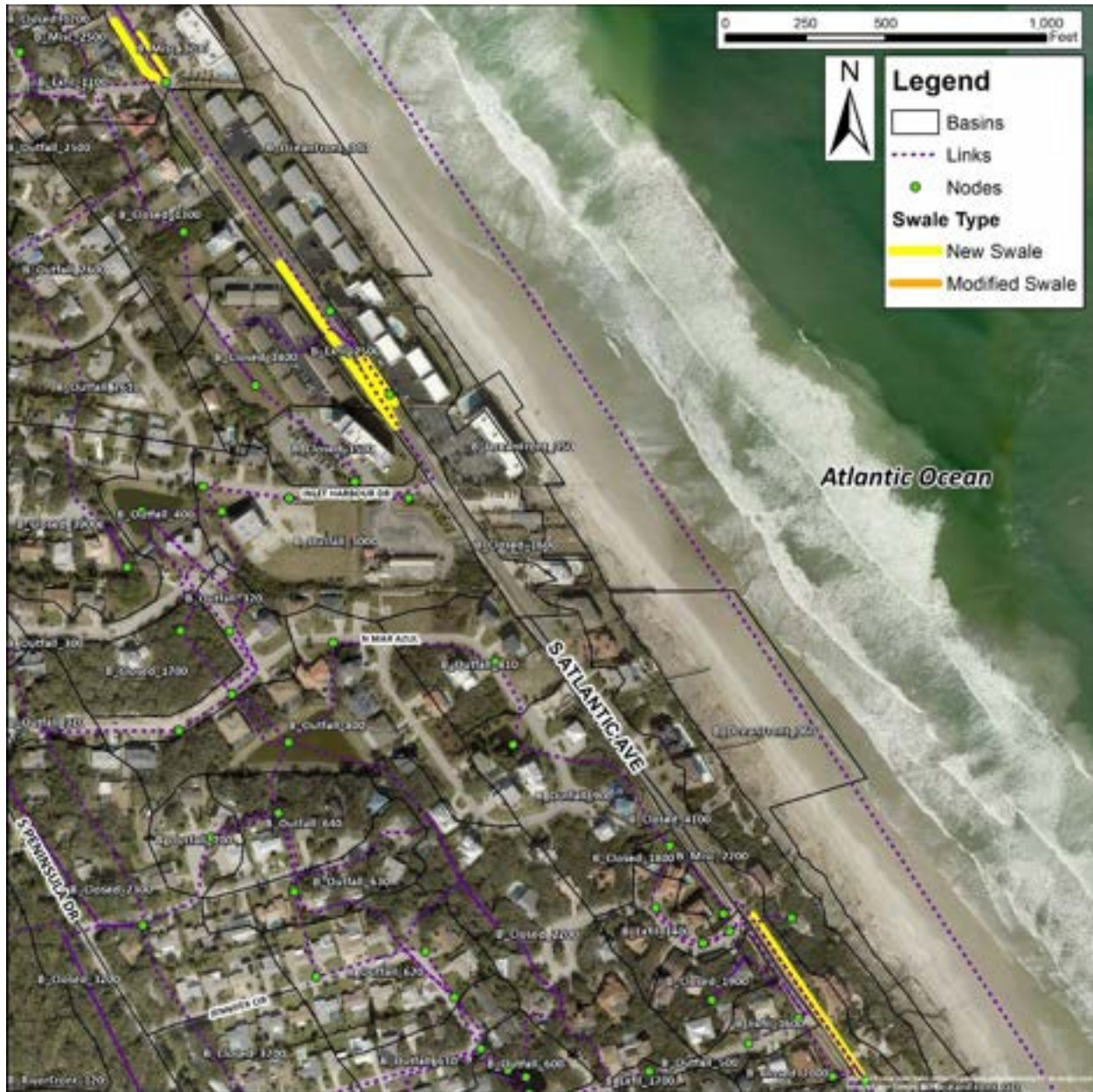
Figure 41. S Atlantic Avenue Additional Swale Locations Between Glenview Avenue and Beach Street
