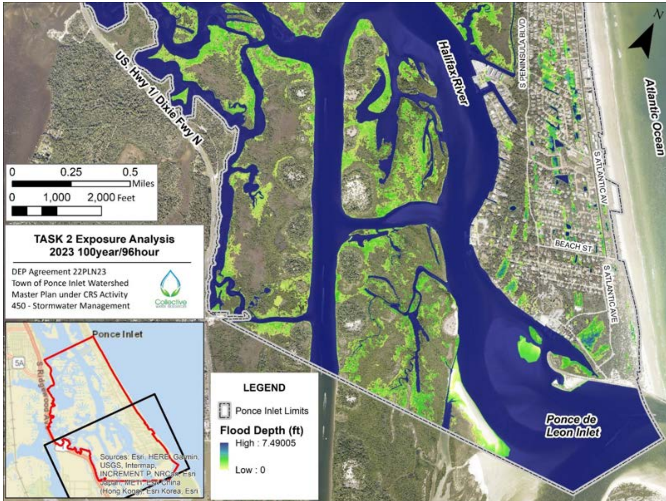
Figure F10 Stormwater Exposure 2023, 100year/96hour design storm South
