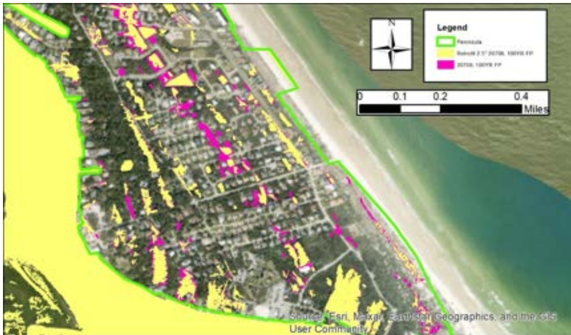
Figure 35. 2070 IL Floodplain with 2.5-Inches of Retrofit Retention/Storage
